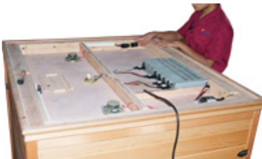
FIG-14 Connectors on the internal top board
