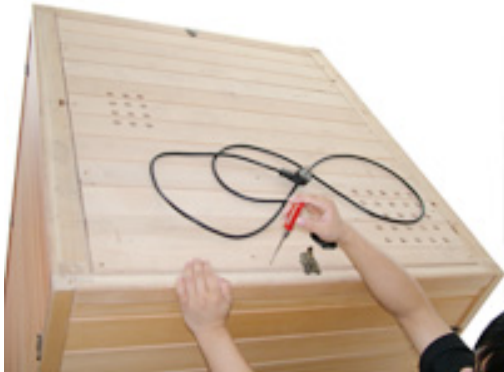
FIG-23 Fix the external board with screws
